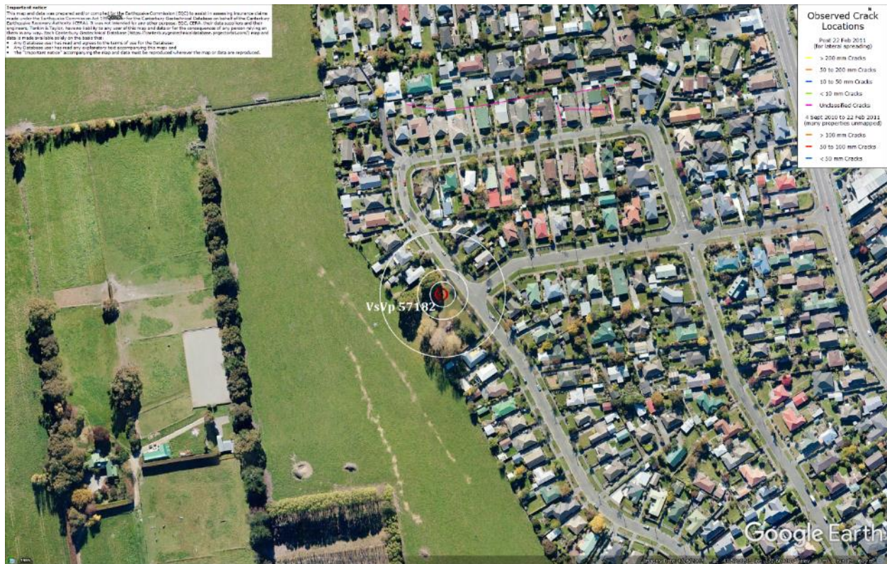
Figure 26: Absence of cracks indicating no lateral spreading for Canterbury Earthquake Sequence.
